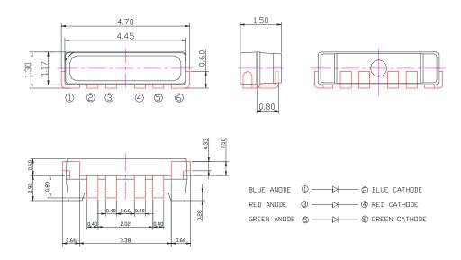
Tolerance of measurement of the dimension is  $\pm 0.1$
