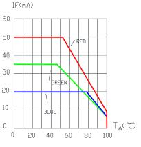
MAXIMUM FORWARD DC CURRENT VS, AMBIENT TEMPERATURE.
