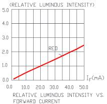
The above data are collected from statistical figures that do not necessarily correspond to the actual parameters of each single LED. Hence, these data will be changed without further notice.
