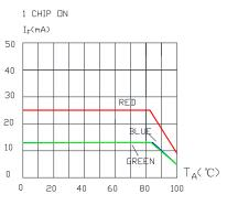
MAXIMUM FORWARD DC CURRENT VS, AMBIENT TEMPERATURE.
